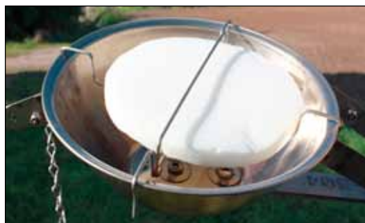
Abb. 16: Sammelmedium Sorbent Impregnated Polyurethane Foam Disk (SIP)
