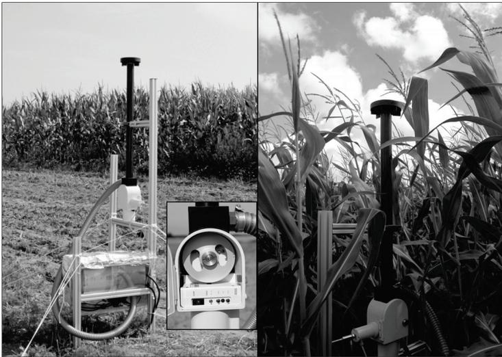
Fig. 1: The new pollen monitor PMO, a high-volume sampler with omni-directional inlet for continuous measurement of pollen concentration in the air even under turbulent conditions like inside of maize fields in canopy height or close to the field.
